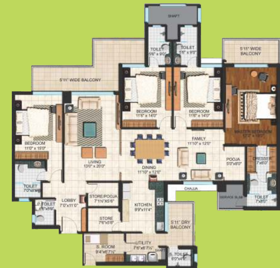
▪ Built-Up Area - 2572 Sq. Ft. ▪ Super Area - 3008 Sq. Ft. 4 BHK 2nd, 3rd, 4th, 5th, 10th, 11th, 12th, 13th Typical Floor Plan Without Corner Balcony
