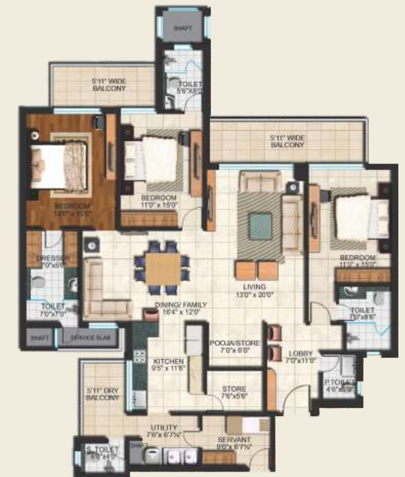
▪ Built-Up Area - 2082 Sq. Ft. ▪ Super Area - 2491 Sq. Ft. 3 BHK 6th, 7th, 8th, 9th, 14th Typical Floor Plan
